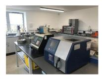
Our fully equipped TASCC laboratories in Chichester and Shoreham provide us with all the information we need to maximise the marketing of your grain. Our FOSS Infratec NIR grain analysers are calibrated using the industry standard ring-testing against 37 laboratories from six continents ensuring unparalleled levels of accuracy during testing.
